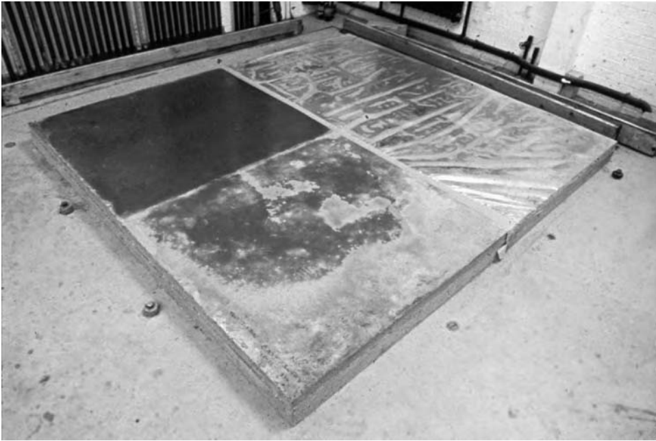
Figure 12.2 Curing methods: acrylic resin on left, polyethylene sheeting on right, no curing (air drying) at bottom
